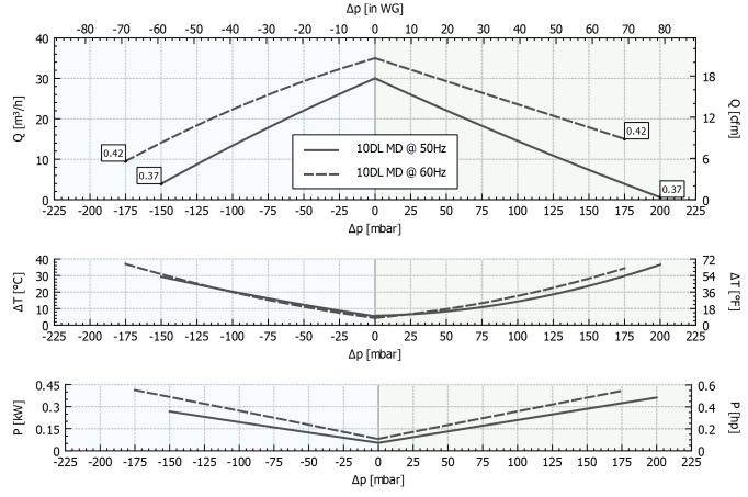
Tolerance on indicated values ± 10%. Data subject to change without notice. Curves referring to air at a temperature of 20 °C and atmospheric pressure of 1013 mbar (abs).
