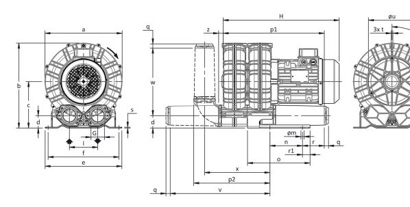
Configuration with a vertical silencer is only available with the CK accessory kit; for all assembly options refer to FPZ. Dimensions in mm NOT Binding
